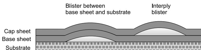
Figure 1. Blistering locations in modified bituminous membranes
