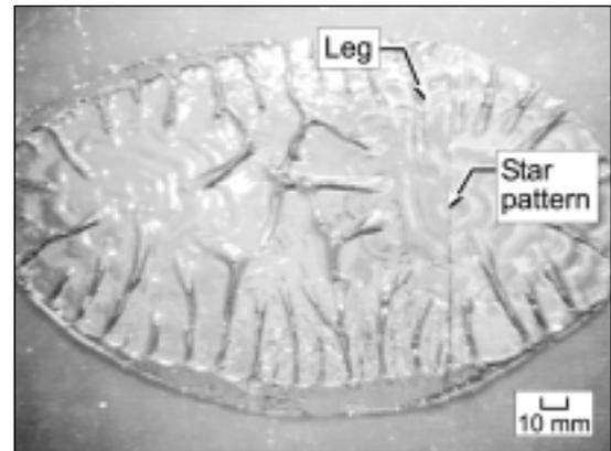
**Figure 4.** Uncoated spots are potential origins of blisters.
