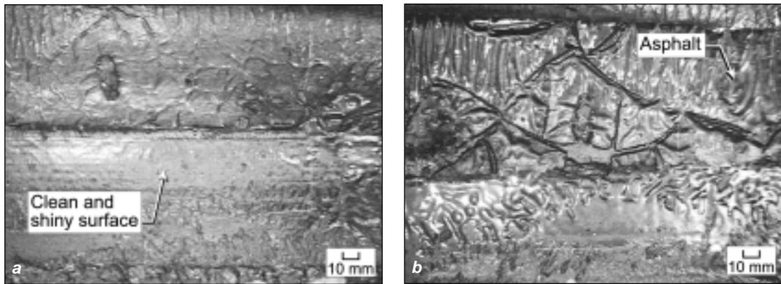
**Figure 2.** Poor interply bonding due to low application temperature
